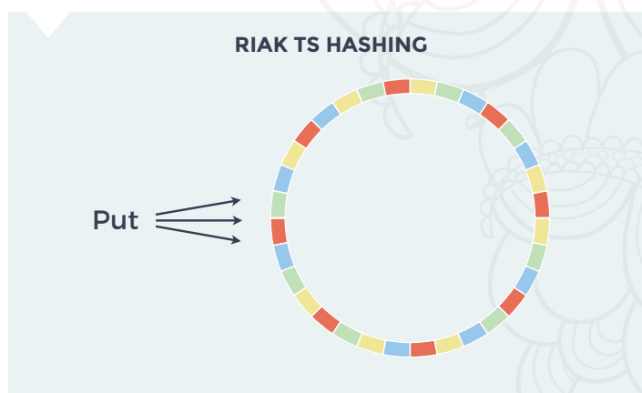
Fig 2: Shows data from the same quantum is written to the same partition. Queries for the time series data from the same quantum are read from the same partition for faster access and faster queries
